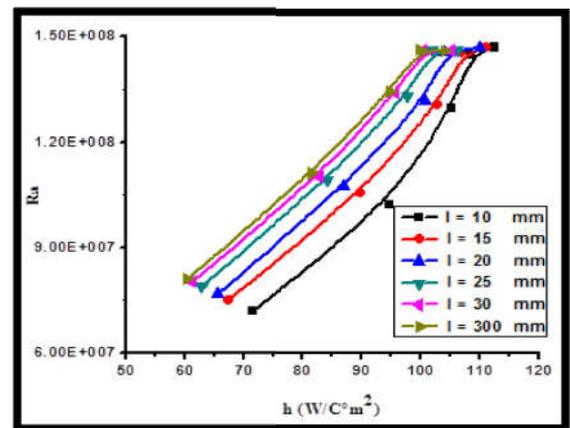
Figure 10 The influence of heat transfer coefficient difference on Rayleigh number at various fin length.
