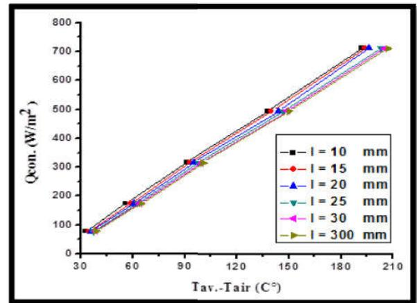
Figure 6 The influence of temperature difference on heat transfer rate at different fin length.
