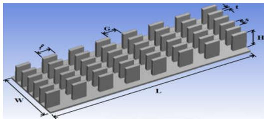
Figure 1 The fin geometry.
