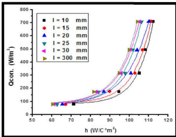
Figure 8 The influence of convection coefficient on heat transfer rate at different length of fin.
