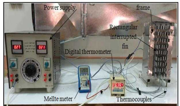
Figure 4 Photograph of the experimental RIG with the measuring instruments.
