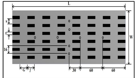
Figure 3 The location of thermocouples on the testbed.
