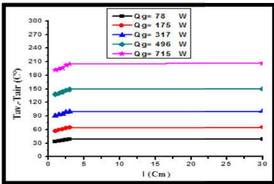
Figure 5 The influence of temperature difference on fin length at different heat flux.
