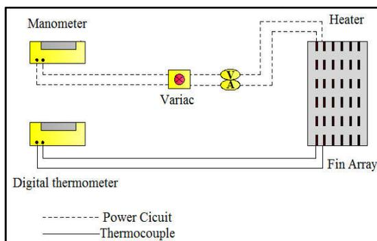
Figure 2 sketch of the electrical circuit.
