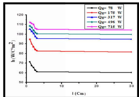
Figure 11 The influence of heat transfer coefficient on length of fin at difference heat flux.
