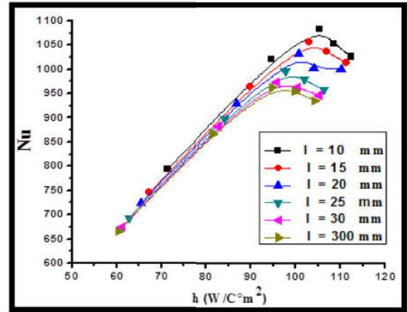
Figure 9 The influence of convection heat transfer coefficient on Nusselt number at difference fin length.
