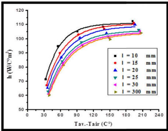
Figure 7 The influence of heat transfer coefficient on temperature different at varies fin length.
