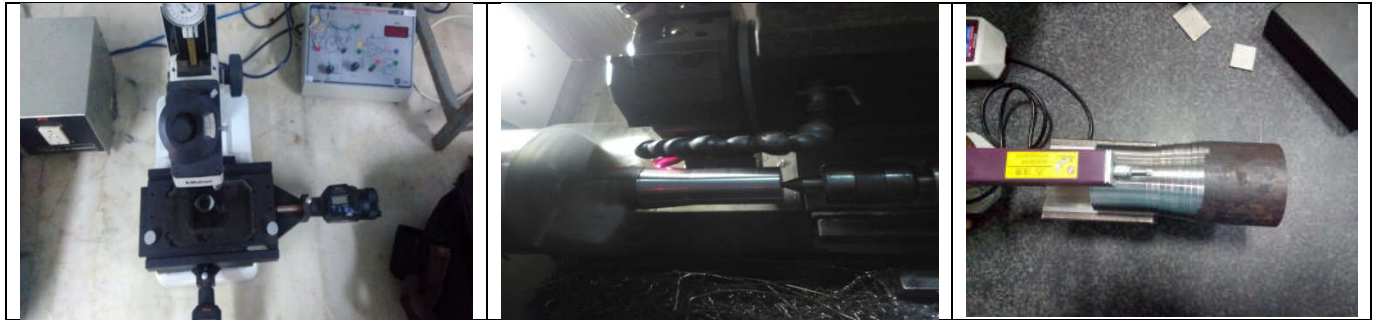
Figure 2 Tool Wear, Interface Temperature and Surface Roughness measuring setup
