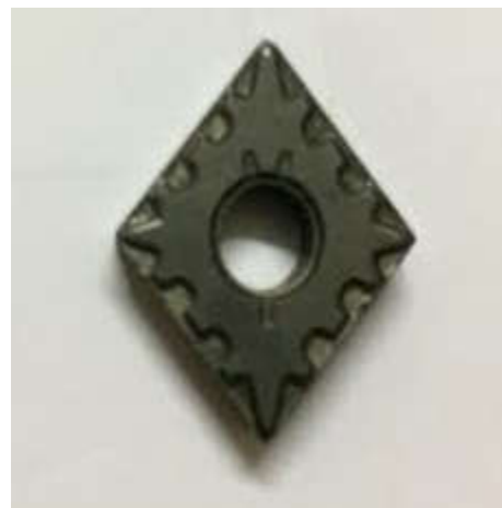
Figure 1 Multi-layer Al-Ti-N coated carbide insert using Thermal Evaporation Technique
