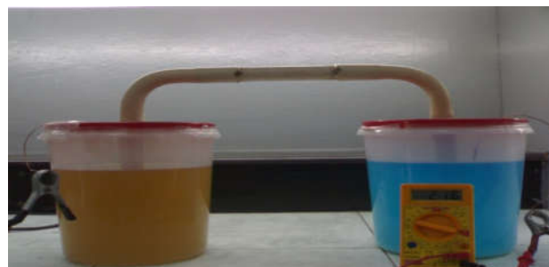
Figure 1 Simple model of a Microbial fuel Cell
