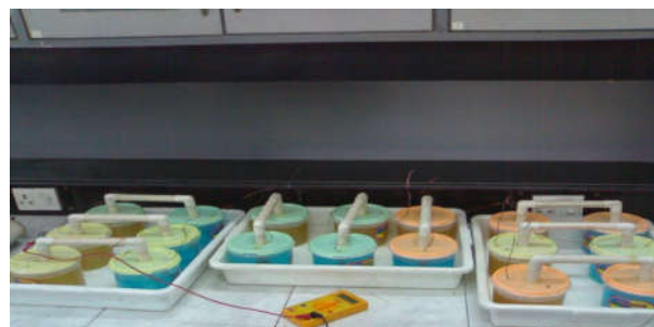
Figure 2 Arrangement of MFCs in series
