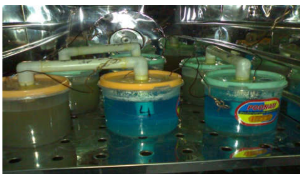
Figure 4 MFCs for permeabilizer effect testing placed in incubator
