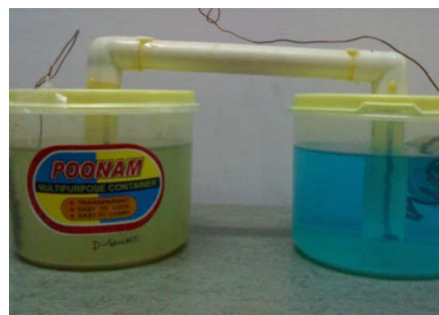
Figure 2 Extra-C MFC with wastewater as the nutrient source
