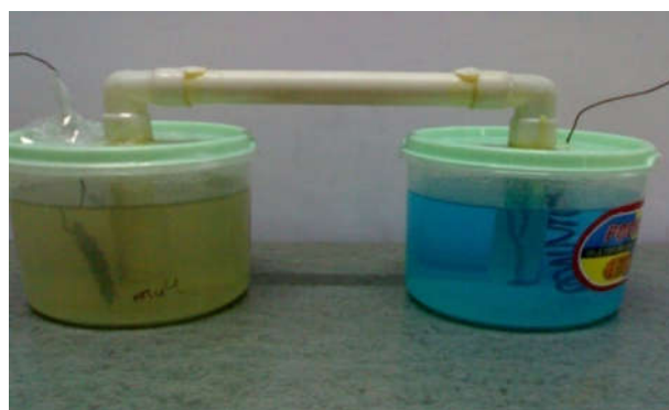
Figure 3 Extra-N MFC with wastewater as the nutrient source
