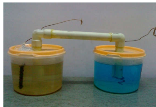
Figure 1 Normal MFC with wastewater as the nutrient source
