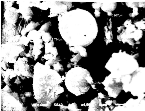
Fig 1 SEM picture showing particle size of cement
