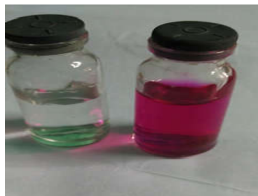
Pink colour : Positive Rapid urease test No change in colour: Negative Rapid urease test
