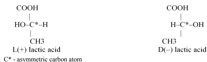
Fig 1 Structure of D and L Lactic acid
