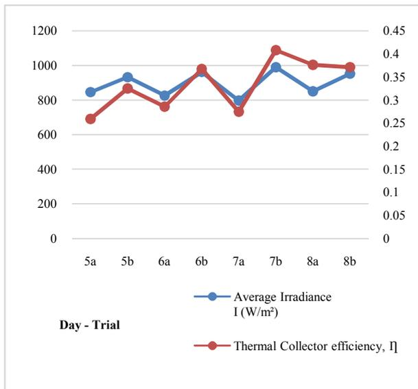
Fig 7 Variation of average irradiance and thermal collector efficiency for four days (with partition setup)
