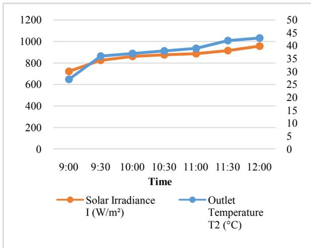
Fig 2 Variation of solar irradiance and outlet temperature with time for day 1 trial 1
