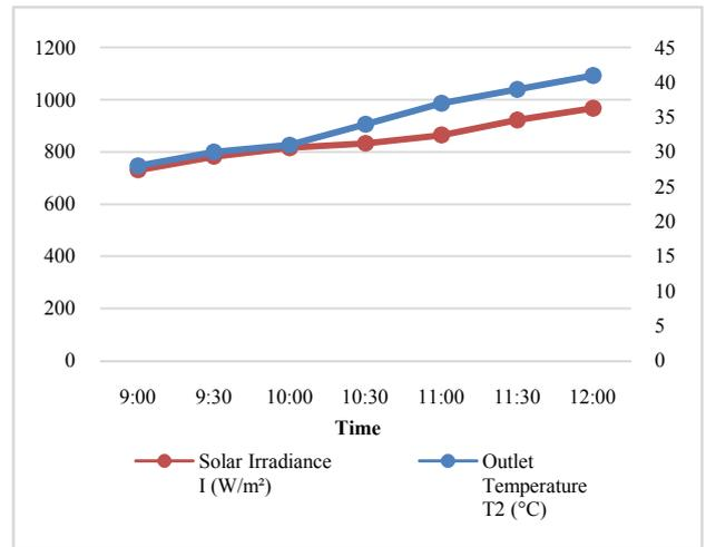
Fig 4 Variation of solar irradiance and outlet temperature with time for day 5 trial 1
