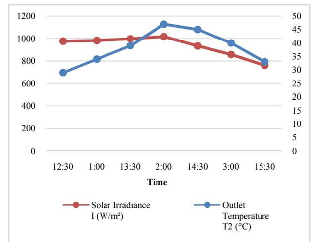
Fig 5 Variation of solar irradiance and outlet temperature with time for day 5 trial 2
