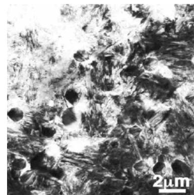
The above figure shows the cracking section of die at 2micron range where the die is made of material D6 at final breakdown with double cycle stroke of crack edge for SEM analysis. By observing the above SEM image some ductility and non-elasticity observed in this. After the crack propagates at the damage section after second preheat with 500 strokes the property of elasticity has to regain for carbon deposit after heating.
