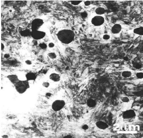
The above figure shows the cracking section of die at 2micron range where the die is made of material D6 at initial breakdown at the second area of heated die. This shows the application of necessity in case study of various components dies which is having complexity.
