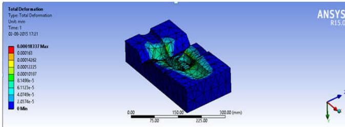
The deformation formed at the walls of the impression with multiple cycles of impact. After the impact of 100 cycles the deformation will be 0.01 at cold condition of one pre heat. By random checkup of getting deviated deformation applicability will be more in hot condition which described in previous research paper i.e. 0.1mm in cycle
