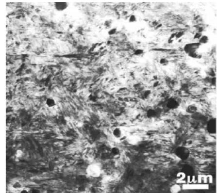
The above figure shows the cracking section of die at 2micron range where the die is made of material D6 at initial breakdown with pre heat treatment after 100 cycles of hammer strokes. In the SEM analysis we observed the carbon deposits with some porosity problems because of unusual and conventional process of pre-heating.
