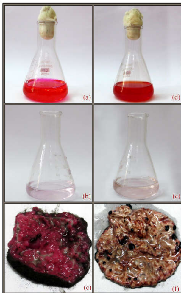
Figure 3 Initial colour of medium containing (a) rose Bengal (d) congo red (b,e) Clear solution after incubation with Aspergillus niger on 10th day and (c,f) fungal mat showing adsorption of (c) rose Bengal (f) congo red.
