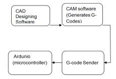
The circuit to be printed is designed on Eagle(CAD) software, whose output is a gerber file in .DXF format. This drawing is then fed to the FLAT-CAM which is a CAM software whose output is G-code in .NC format readable by the machine.
