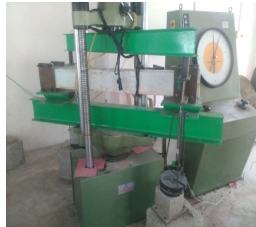
Figure 2 a Torsion test setup
