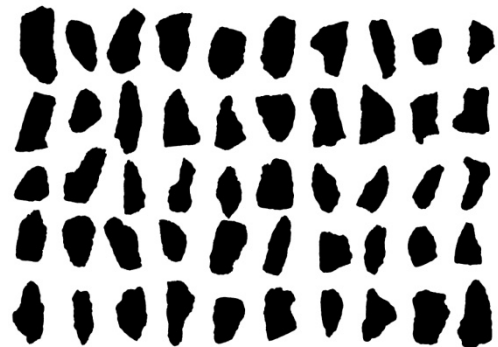
b Processed image of C_{13.2r} aggregate
