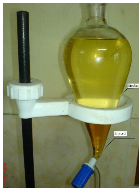
Fig 1 After Base esterification
