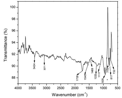
Fig 6 FTIR spectrum of GTCAZS crystal.
