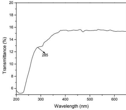
Fig 3 UV-VIS transmission spectra of GTCAZS crystal.
