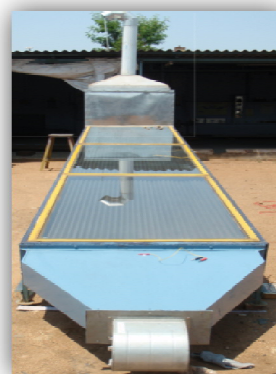
Fig 1 The entire unit with solar air heater, a dryer and a storage chamber
