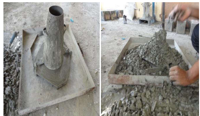
Fig 3 Slump cone and collapse of concrete after lifting
