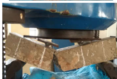
Figure 2 Compressive Strength and Flexural Strength Testing
