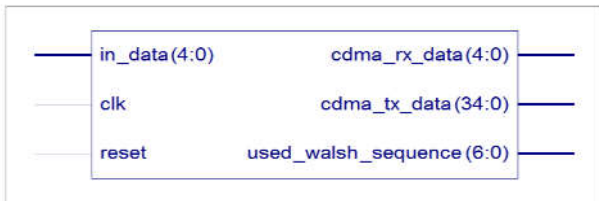
Figure 5 Here Clock, Reset signal applied with input data and Gives Receiver output when applying Walsh Sequences.
