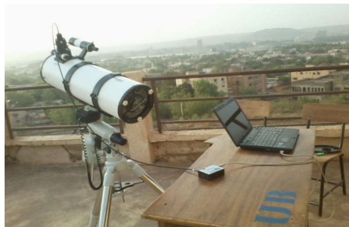
Figure 2 Photo of the MAX-DOAS measurement device on the roof of the FST "Block B" building.
