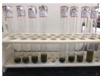
Figure 15 Synthesis of iron nanoparticles (0.01M of FeCl 3 in used C.sinensis leaf extracts)
