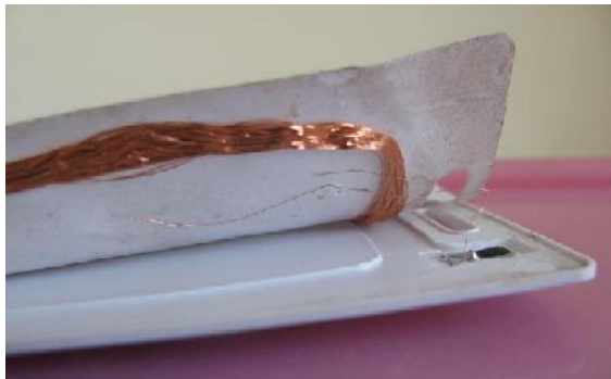
Fig 2 Removing The Backside Layer Of The Tag Discloses The Above Look.
